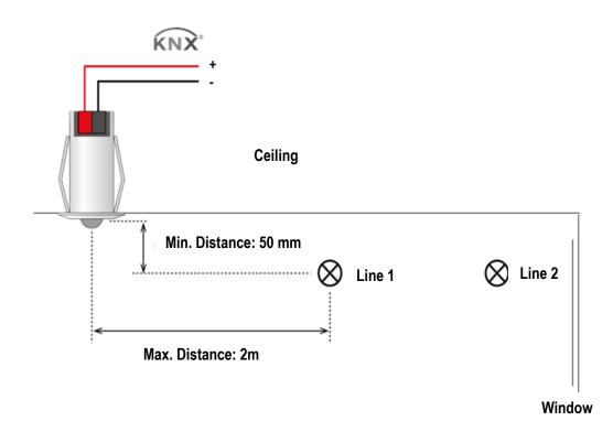
Focus the sensor for brightness measurement:
