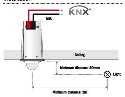
**IMPORTANT:** Connecting the KNX bus upside down causes damage to the equipment
