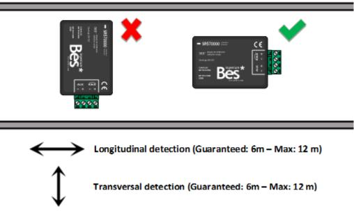
The detection area (placing the SR570000 at 2.5m from the floor) is:
